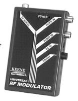
standard aerial input; it can also be used to feed the signal from a TV surveillance camera into a domestic cable installation.
